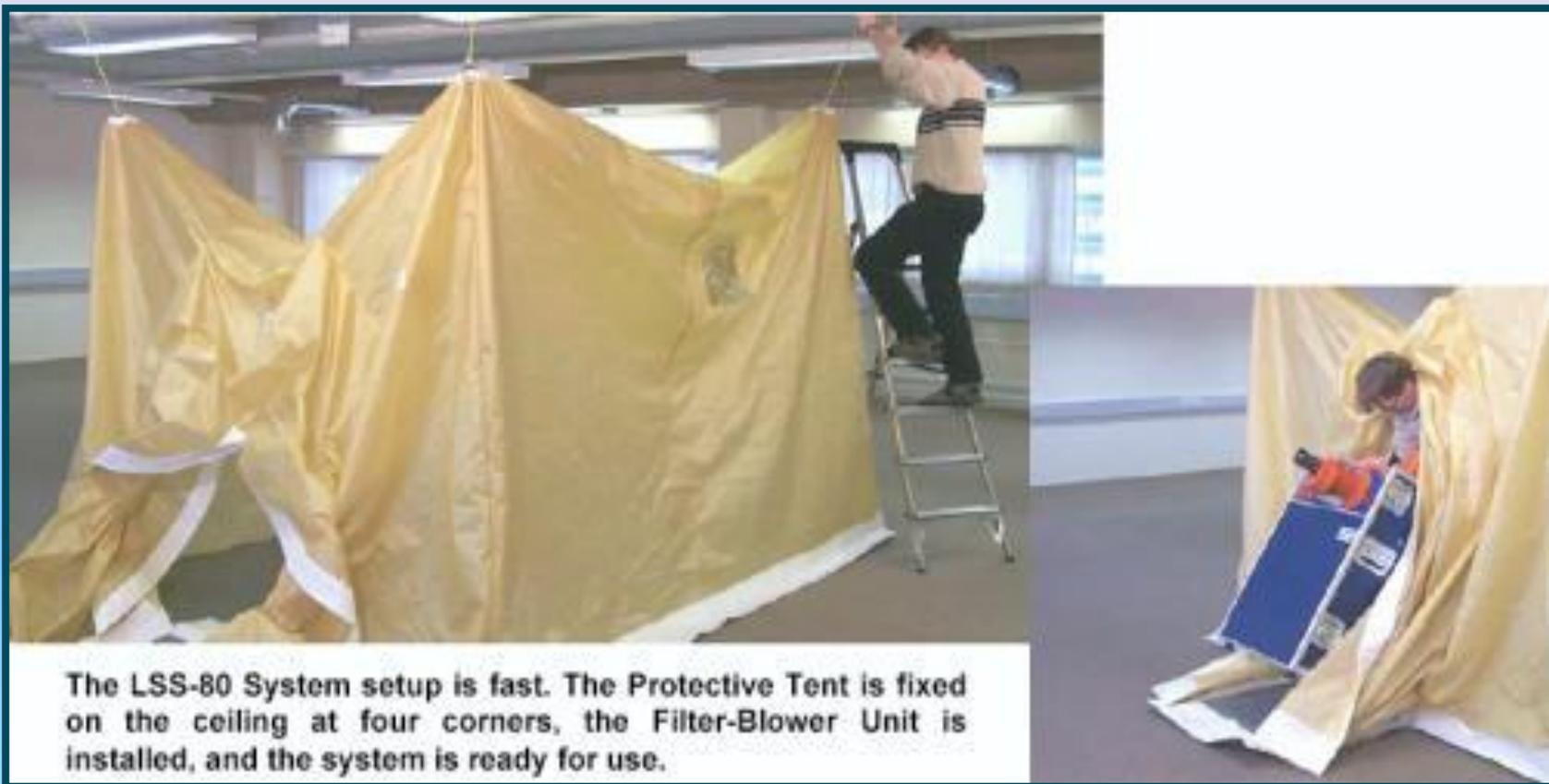
The LSS-80 System setup is fast. The Protective Tent is fixed on the ceiling at four corners, the Filter-Blower Unit is installed, and the system is ready for use.
